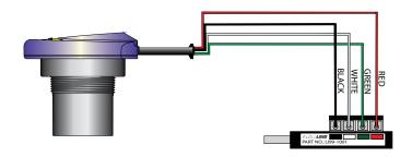
\* Once EchoSonic II is configured, isolate the white and green wires from active power to prevent a short of the configuration circuit
