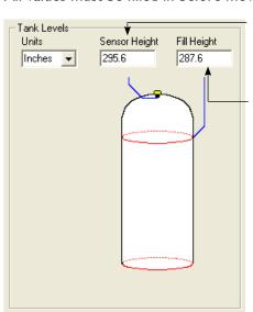
Sensor Height: Distance from the bottom of the tank to the bottom of the transducer
