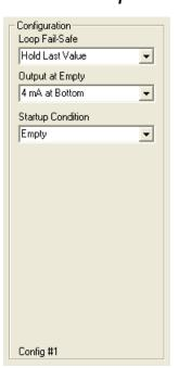
This section of WebCal is where you select the application's configuration settings. Start from the top and work to the bottom, choosing the selections that are applicable to your configuration. "Not Applicable" will automatically show when a selection doesn't apply to your configuration settings, and you may move on. All configuration settings must be selected or have "Not Applicable" before you can continue to step 2.
